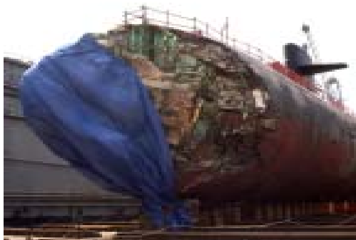
A view of the damage to San Francisco's bow
