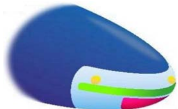
Conceptual drawing of a ceramic hull-adaptable sonar array that will replace the standard hull array
