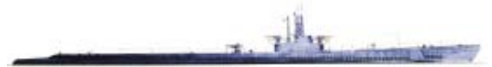
A profile view of late war fleet boat showing the upgraded anti-aircraft armament
