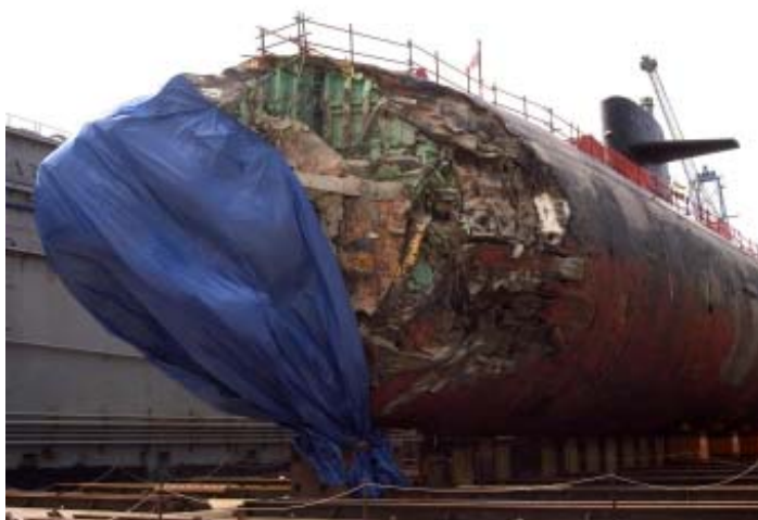
San Francisco's damaged bow, definitely in need of replacement
